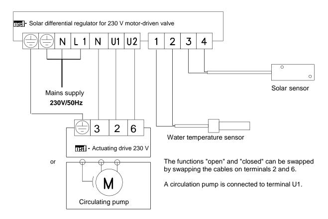
If actuating drives from other manufacturers are used, please observe the wiring diagram supplied with the actuating drive!
